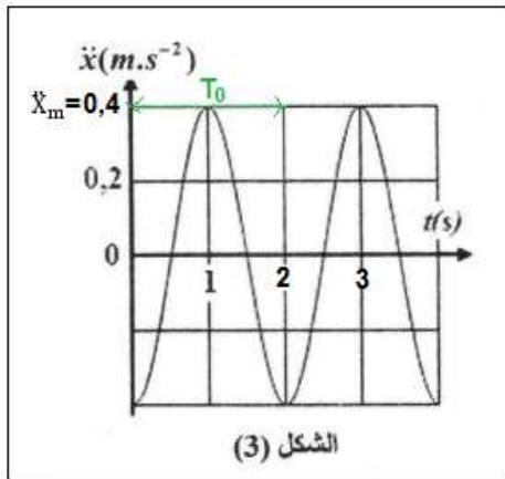
$$\ddot{X}_m = \frac{\ddot{X}_m}{\left(\frac{2\pi}{T_0}\right)^2} = \frac{\ddot{X}_m \cdot T_0^2}{4\pi^2}$$
