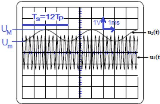
$$12T_p = 4 \text{ div} \times 2 \text{ ms/div} \Rightarrow T_p = \frac{8 \cdot 10^{-3} \text{ s}}{12} = \frac{1}{1500} \text{ s}$$
