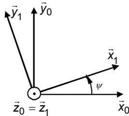
$$V_{1/0} : \left\{ \begin{array}{l} \vec{\Omega}_{1/0} = r_{1/0} \vec{z}_0 = \dot{\psi} \vec{z}_0 \\ \vec{V}(G \in 1/0) = w_{1/0} \vec{z}_0 = \dot{z} \vec{z}_0 \end{array} \right\}$$
