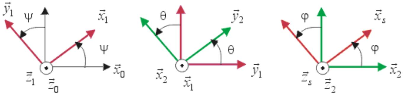
$$B_0(\vec{x}_0, \vec{y}_0, \vec{z}_0) \xrightarrow{(\psi, \vec{z}_0)} B_1(\vec{x}_1, \vec{y}_1, \vec{z}_1) \xrightarrow{(\theta, \vec{x}_1)} B_2(\vec{x}_2, \vec{y}_2, \vec{z}_2) \xrightarrow{(\varphi, \vec{z}_2)} B_S(\vec{x}_S, \vec{y}_S, \vec{z}_S)$$
