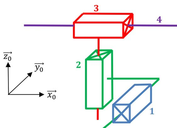
$$\{\mathcal{V}_{4/1}\} = \begin{Bmatrix} 0 & U_{4/3} \\ 0 & V_{2/1} \\ 0 & W_{3/2} \end{Bmatrix}_{\mathcal{B}_0} = \begin{Bmatrix} 0 & U_{4/1} \\ 0 & V_{4/1} \\ 0 & W_{4/1} \end{Bmatrix}_A$$
